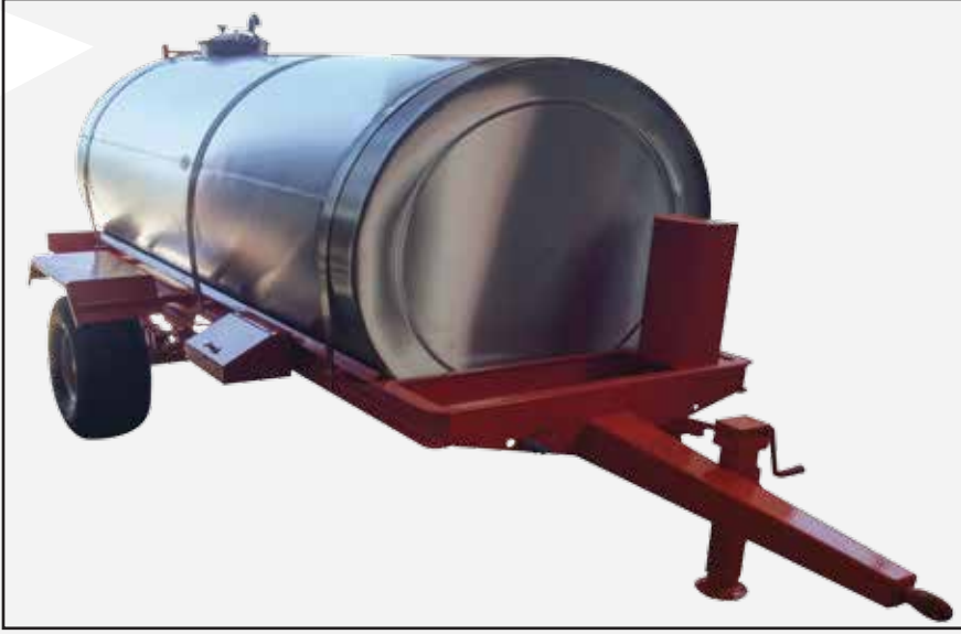
Dingilli Krom Nikel Su Tankı / Axle Chrome Nickel Water Tank
